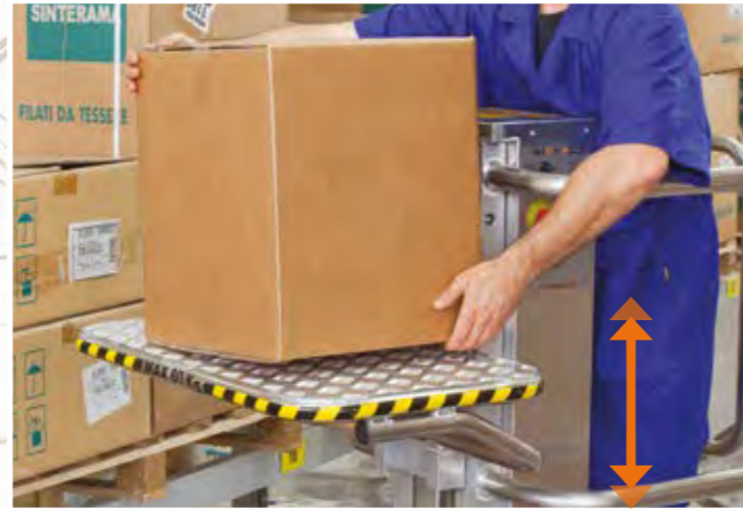
A large loading platform which can be adjusted automatically when raised.
